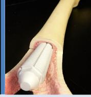
The ScrewLOCK shown in an open femur demonstrating the position of the device.
